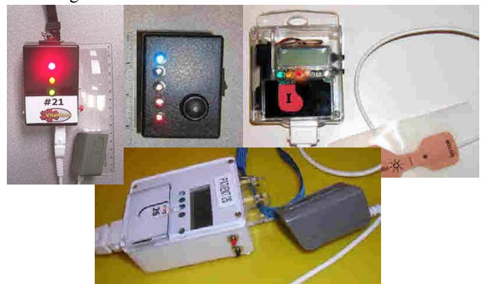
Fig 8: An Iterative Package Design. From left to right, black Mote 21 is the initial prototype with three LED lights. The black mote with five LED lights and buzzer is prototype number two. Prototype number three is a clear mote with a LCD screen to display the oxygen saturation and heart rate. The photo-interrupter cards are displayed in prototype 3. The final prototype is the white mote with the LCD screen and push buttons.
