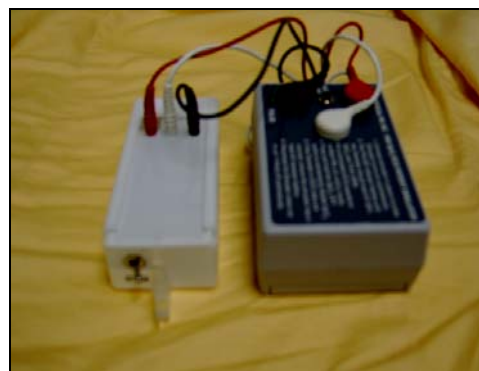
Fig. 3. Embedded EKG device prototype to collect a patient's heart beat (seen attached to an EKG waveform simulator)
