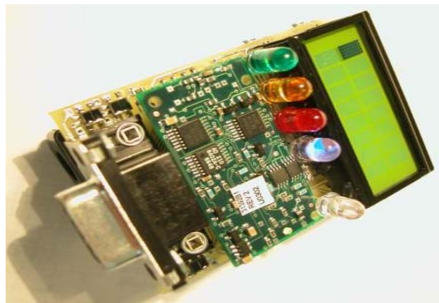
Fig. 1 a) Electronic Triage Tag with pulse-oximeter board attached. b) Architecture of the Electronic Triage Tag (includes MicaZ mote and AID-N custom built Etag board).
