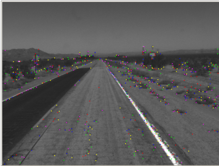
Figure 8: Tracking output, sample frame, obtained with selections in figure 7 as input. Tracks are displayed as dots of different colors, their total number in this frame is 562. The sequence is available at http://www.cs.ucla.edu/~bissacco/jpltrack/fpgatrack.mov , together with the results of tracking using the Harris selector http://www.cs.ucla.edu/~bissacco/jpltrack/harristrack.mov
