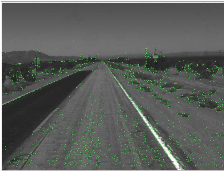
Figure 7: FPGA selection output, sample frame. There are 1162 feature selected, obtained with threshold parameter \lambda_t = 50 . The sequence is available at http://www.cs.ucla.edu/~bissacco/jpltrack/fpgaselect.mov
