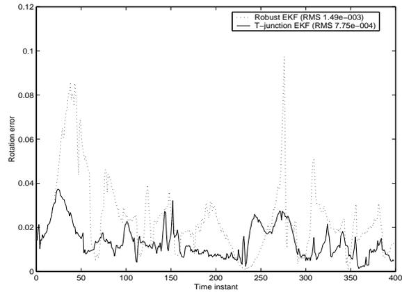
Figure 6: Estimation error of camera rotation for a robust EKF (dotted) and the T-junction EKF (solid). We plot the norm of the RMS error for each time instant and compute the RMS error for the whole sequence. In both cases we can see that the T-junctions EKF improves the estimation of rotation when compared to the robust EKF.
