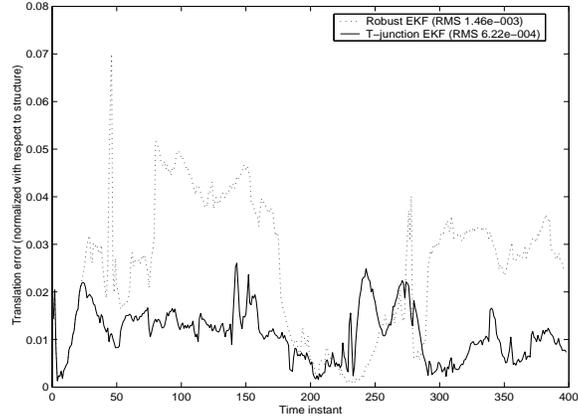
Figure 5: Estimation error of camera translation for a robust EKF (dotted) and the T-junction EKF (solid). We plot the norm of the RMS error for each time instant and compute the RMS error for the whole sequence. In both cases we can see that the T-junctions EKF improves the estimation of translation when compared to the robust EKF.
