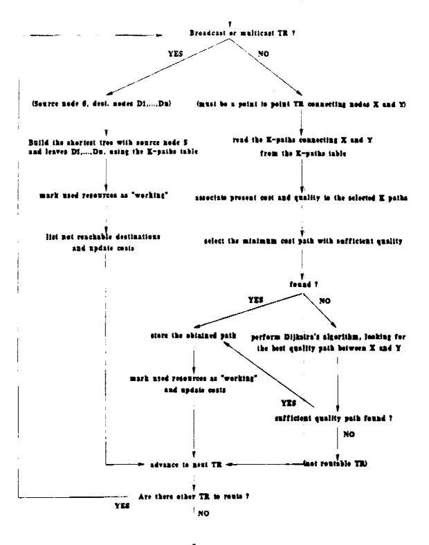
Figure 4: flow chart of the routing algorithm.
