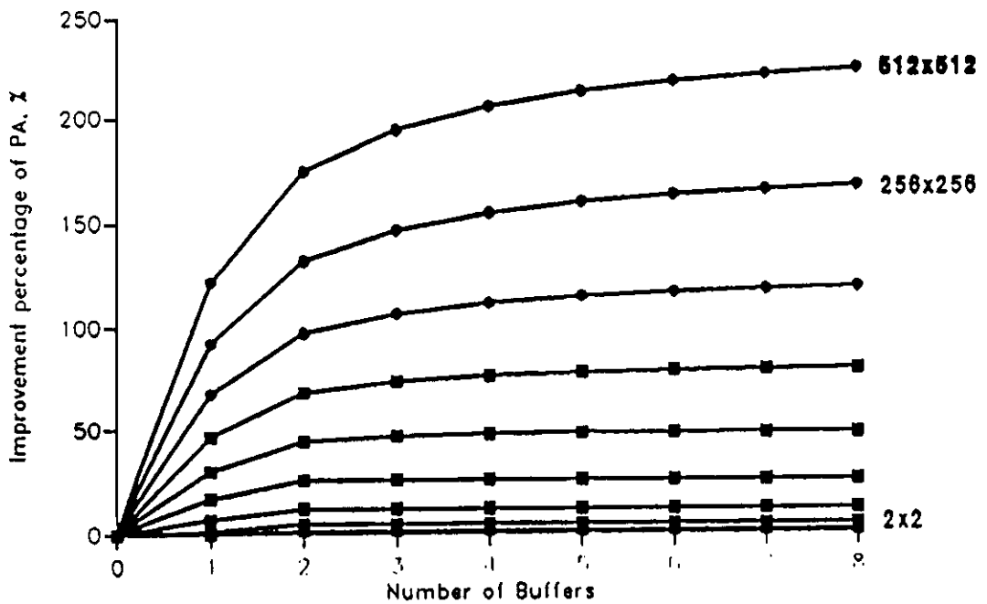
Figure 2.10: The PA improvement percentage by adding buffers for interconnection networks with q=1.0 and a uniform traffic pattern
