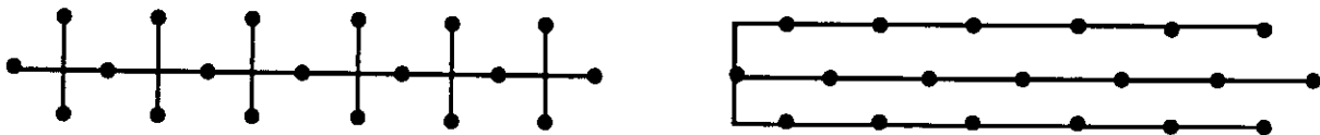
Figure 2: An example where the ratio of a SEPARABLE-MST-derived-RST to the MRST is arbitrarily close to 3/2 . For the pointset shown, the MRST on the left has a cost of (4/3)(N-1) , while any RST derivable from the MST on the right has a cost of 2(N-2) , yielding a ratio arbitrarily close to 3/2 for large enough N .
