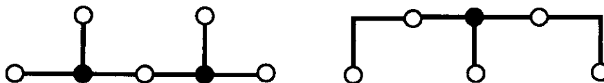
Figure 6b: A 5-point example where the Iterated 1-Steiner performance ratio is 7/6 . The optimal MRST has cost 6, while a possible heuristic output has cost 7.
