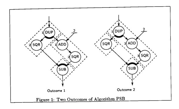
In Figure 1, we see two possible outcomes, depending on which  $v \in succ(s)$  statement 9 choses when s = DUP. In Outcome 1, a result token will appear on the left input of SUB earlier than on the right input, because the left path requires fewer vertices (machine operations) and fewer exposed edges (communication delays) than the right path. In Outcome 2, the two result tokens will appear at SUB at more nearly the same time.
