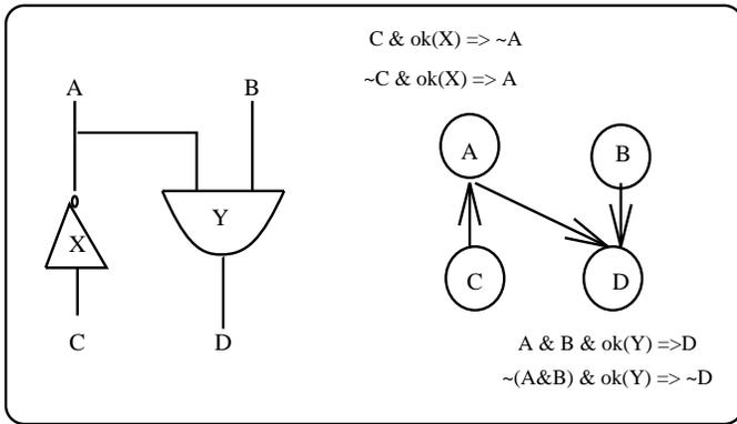
Figure 3: A symbolic causal network describing a circuit.
