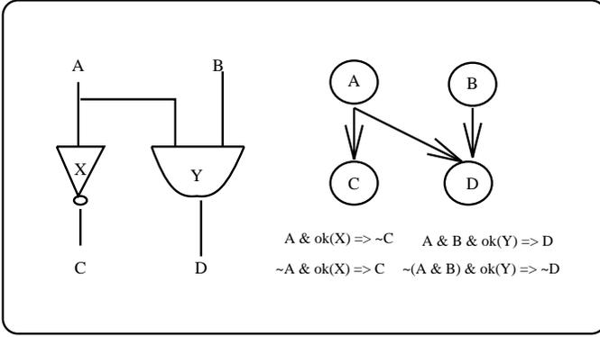
Figure 2: A symbolic causal network describing a circuit.
